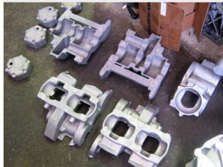
Cast engine casings ready for machining
